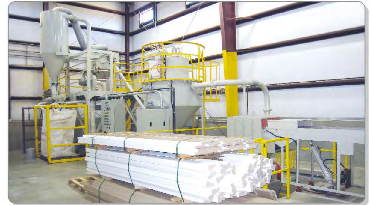
▲ PVC+木粉料從粉碎到磨粉一貫作業流程 PROCESSING OF PVC & WOOD FROM CRUSHING TO PULVERIZING
