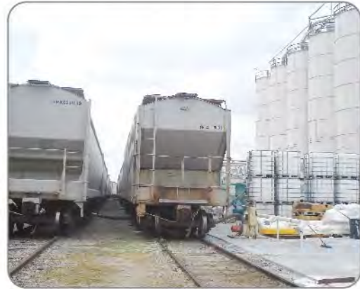
▲ 火車載運管線輸送至SILO TRAIN CONVEYING MATERIAL TO 100-TON SILOS
