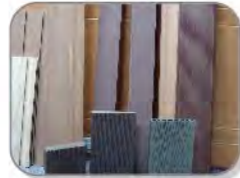
▲ 稻殼、椰子殼或咖啡殼+ 廢料PE製成仿木材 WOOD PLASTIC COMPOUND PROFILES MADE FROM RICE HULL, COCONUT HUSK OR COFFEE SHELL & RECYCLE PE.
