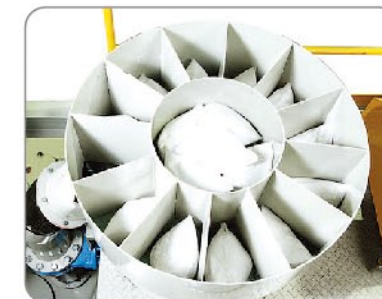
▲ CL-AA 自動投色料設備(一手料一包) INSTALLATIONS OF AUTOMATIC THROWING COLORS (ONE BATCH PER BAG)
